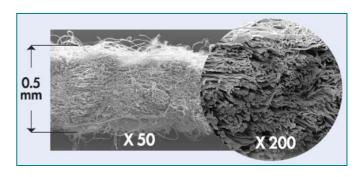
7000 km of microfilaments in 1sqm of Evolon® 100g/sqm lead to an air flow resistance of ~1000 Pa.s/m
