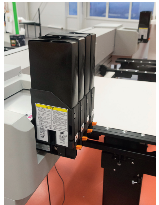
The ink cassettes are refilled using ink bags.
