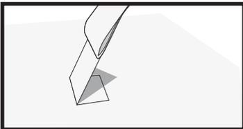
Using a TESA® 7476 adhesive tape, or the like, apply to a surface of 2.5 cm x 5 cm (1 in. x 2 in.) plus some overhang material for easier removal. Fold and promptly tear off perpendicularly to the substrate surface. No traces should remain on the ripped off adhesive tape. Repeat this process in several places.
